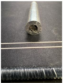
Another error occurred while using the milling tool; I struggled with positioning my part in the vice for cutting and incorrectly used the side face of the mill cutting tool. This left a part of my work rough and a bit jagged, unwanted when attempting to manufacture a utility like a chair. I later understood that allowing the part to extend out from the side of the vice while clamped would have prevented this mistake, and something important to keep in mind when I use a mill in the future.
